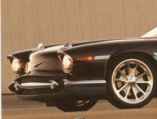
The heart of the 789 is the chassis, suspension, and driveline of a C6 Corvette. Once all the C6 body panels are off, N2A turns it into the sleek, sexy 789. By only changing the skin on the Vette, Kanter's 789 retains all the high-tech safety and performance systems of the donor car.
