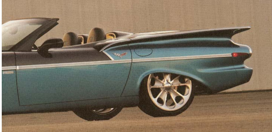
The 789 is a mere 6 inches wider, 6 inches longer, and a scant 50 pounds heavier than a stock C6. Many of the 789's parts are reproduction items from Danchuk, including the headlight bezels and hood bullets.
